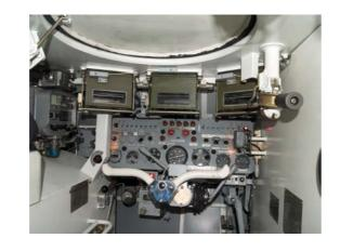
The composition of the equipment and its location in the simulators of the combat compartment and driving compartment correspond to the stations of the vehicle commander, gunner and the driver.
