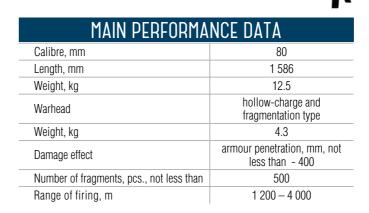
It is intended for firing from B8M and B8V20 rocket pods which are the constituent part of rocket armament of aircrafts like Su-22, Su-24. Su-25. Su-27. MiG-23. MiG-27. MiG-29 and helicopters like Mi-8, Mi-24, Mi-28, as well as for destruction of various types of ground-based targets (tanks, selfpropelled artillery launchers, APC, missile launchers, radar stations, aircrafts on the ground, ammunition depots, special trains, manpower).
