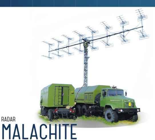
Radar «MALACHITE» - digital, interference-proof radar reconnaissance aircraft and surface targets provides detection, identification of the origin and transmission of radar information consumers automatically. The structure of «MALACHITE» radar includes:
