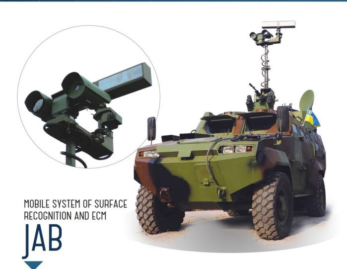
Mobile System of surface recognition and ECM «JAB» is intended for detection, classification and identification of surface moving targets as well as low-speed low-flying air targets, target pointing with the aim to provide performance of tasks on security of wide areas and reconnaissance.
