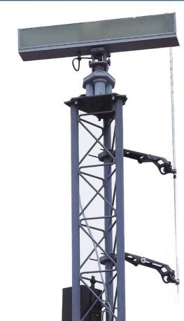
SURFACE AND LOW-FLYING TARGETS DETECTION RADAR 111L1-LIS
