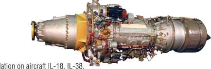
This engine is designed for installation on aircraft IL-18, IL-38, An-8, An-12, An-32, An-32V-200, Be-12 and their versions, which service medium- and long-range routes (up to 6 500 km).
